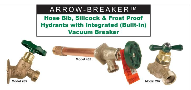
hampion-Arrowhead's complete line of Arrow-Breaker<sup>™</sup> Hose Bibs and Frost Proof Hydrants come with Integrated (Built-In) Vacuum Breakers. The first of its kind. An integral unit, the All-In-One Arrow-Breaker<sup>™</sup> eliminates the need for an ugly "thread-on" vacuum breaker and the associated flow-loss. The Arrow-Breaker<sup>™</sup> is IAPMO listed and in compliance with ASSE standards.
